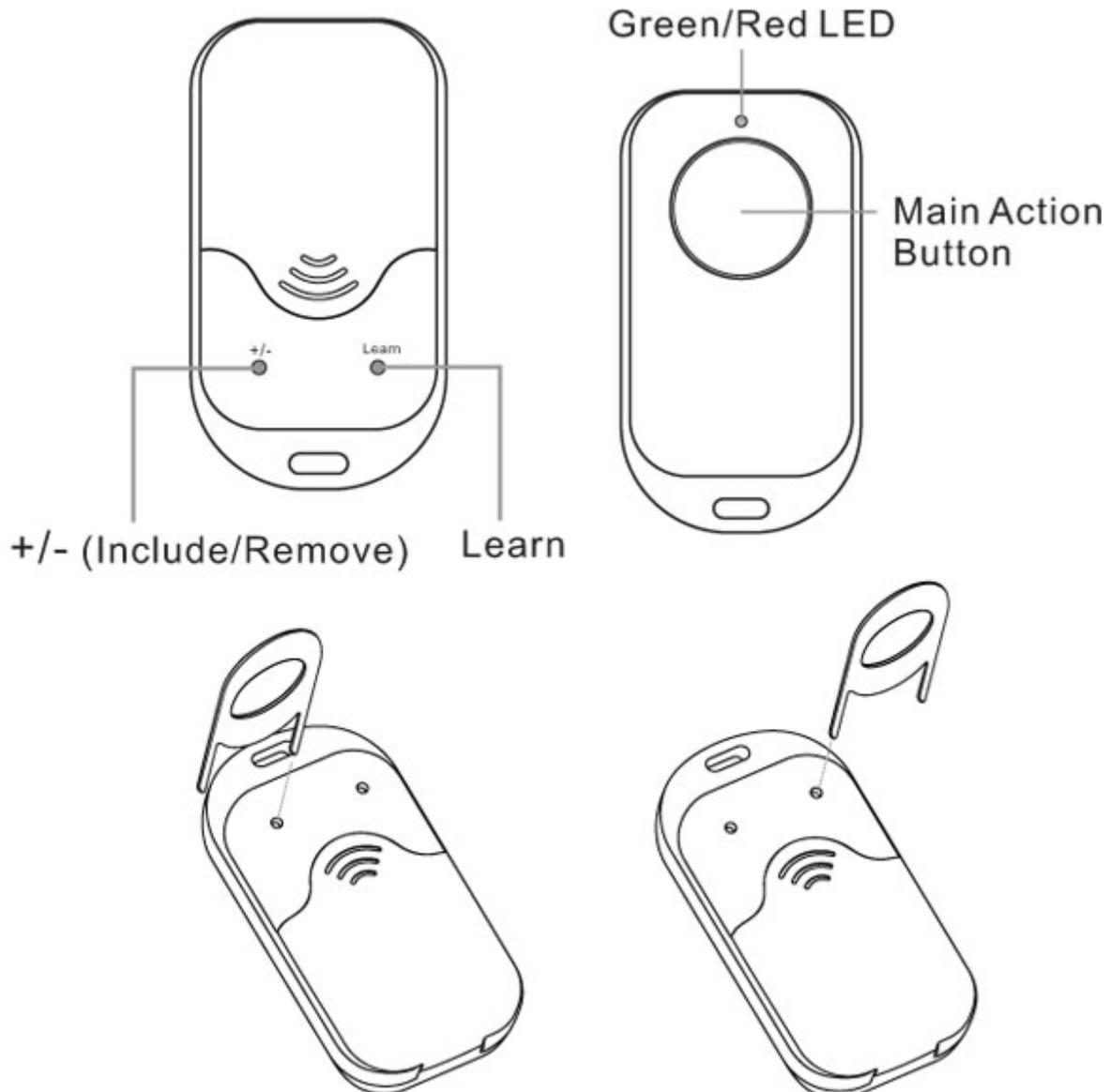
Your Panic Button will now work as a remote control within your Z-Wave network, allowing it to both control associated devices and act as a tool for adding/removing devices to/from your Z-Wave network.
